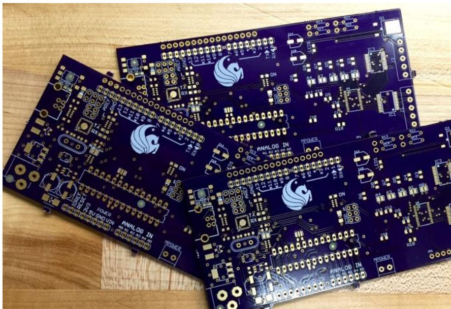
Figure 28 – UCF Custom Printed Circuit Board from OSHPark
